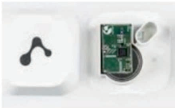
Figure 5: Beacon ouvert Kontakt.io 55*55*15mm [6]
